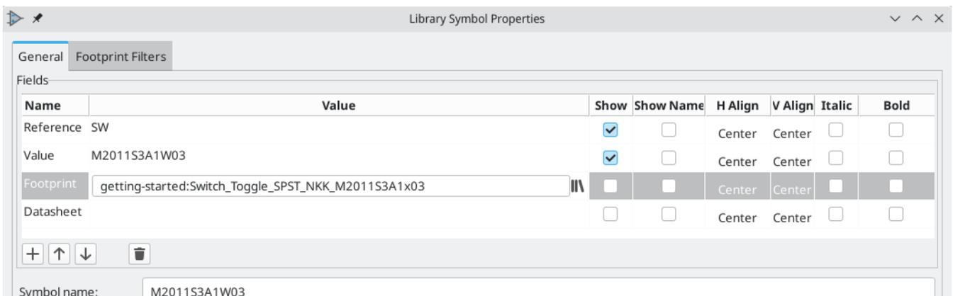
Symbols can specify a preselected footprint. Footprints do not need to be manually assigned to such symbols, because a footprint was chosen when the symbol was created. Users can override the preselected footprint during the footprint assignment process as normal. Defining a default footprint is a good idea for
