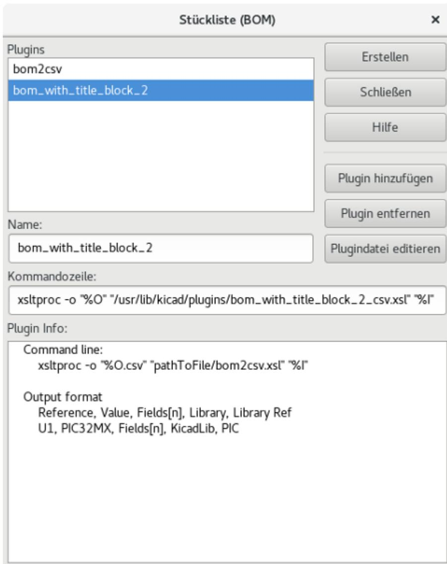
Additional scripts can be added to the list of BOM generator scripts by clicking the **+** button. Scripts can be removed by clicking the **🗑** button. The **🖋** button opens the selected script in a text editor.
