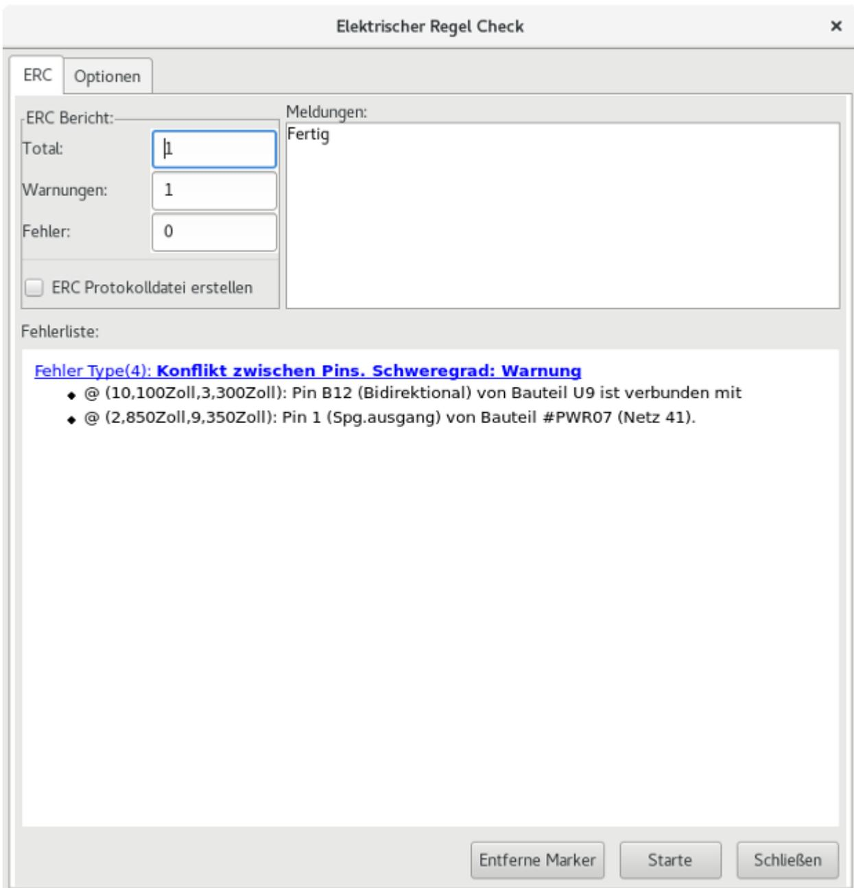
Any warnings or errors are reported in the **Violations** tab, and markers for each violation are placed in the schematic so that they point to the relevant part of the schematic. Warnings are indicated by yellow arrows, and errors have red arrows. Excluded violations are shown as green arrows. A list of the ignored tests are shown in the **Ignored Tests** tab. A report file in plain text format can be created after running DRC using the **Save...** button.
