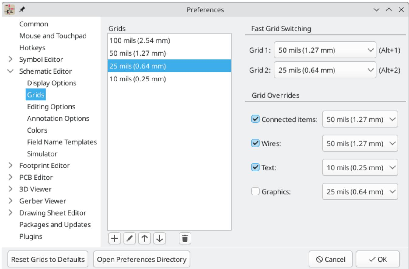
In this dialog you can select an active grid from the list of grids, reorder the list of grids ( $\uparrow$  /  $\downarrow$ ), and add ( $+$ ), remove ( $\text{trash}$ ), or edit ( $\text{pencil}$ ) grids. Grids defined in this dialog can have unequal X and Y spacing as well as an optional name. The grid spacing and name are specified when you create or edit a grid.
