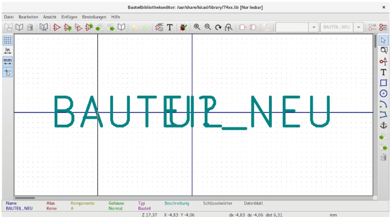
The blue cross in the center is the symbol anchor, which specifies the symbol origin i.e. the coordinates (0, 0). The anchor can be repositioned by selecting the button and clicking on the new desired anchor position.
