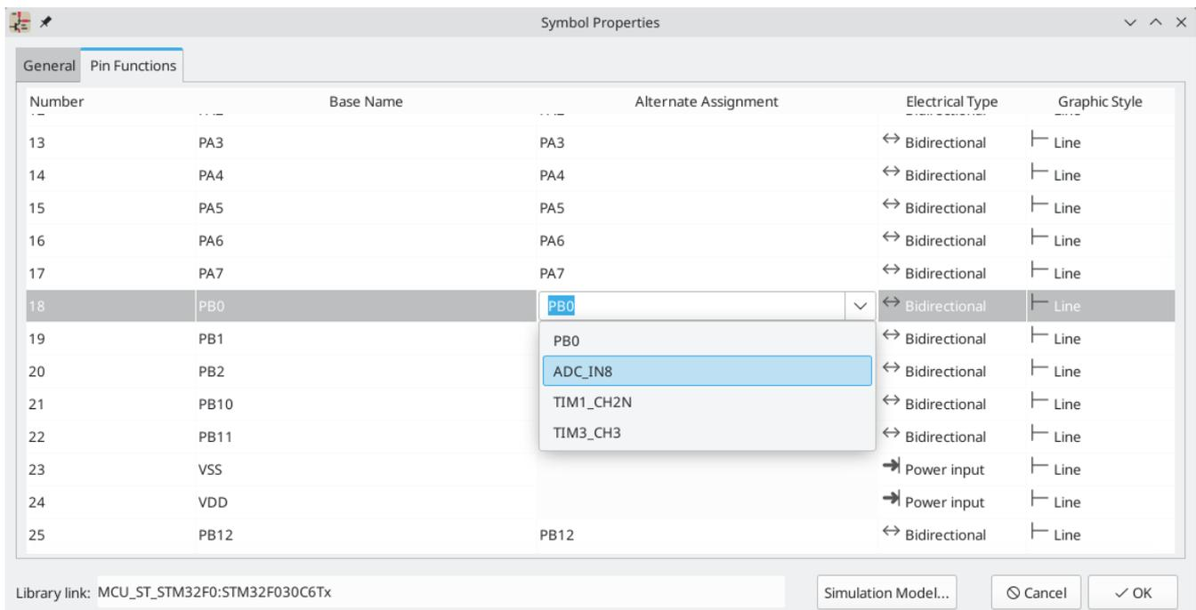
Pins that have alternate functions available are displayed with a small graphical indicator next to the pin name, as shown in the screenshot below. To globally show or hide these indicators, use **View** → **Show Pin Alternate Icons**.
