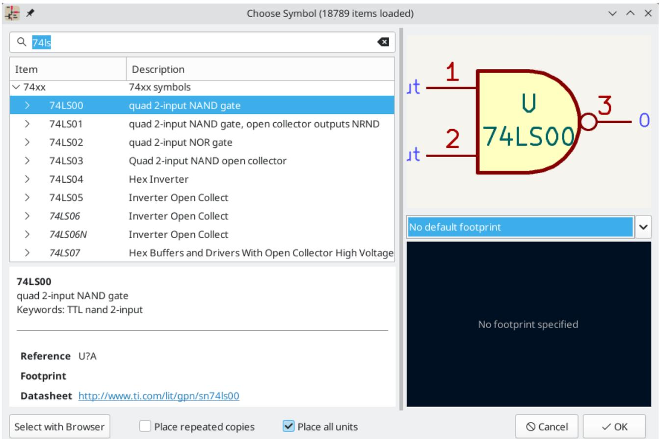
By default, only the symbol/library name and description columns are shown. Additional columns can be added by right-clicking the column header and selecting **Select Columns**.
