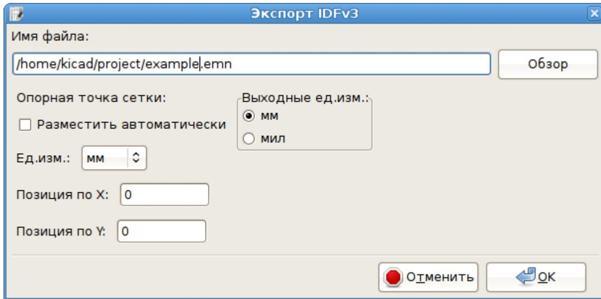
**Grid reference point:** Choose where the exported model's reference point should be. If the **Adjust automatically** option is selected, KiCad will set the reference point to the centroid of the PCB. Otherwise, the reference point is set relative to the display origin.
