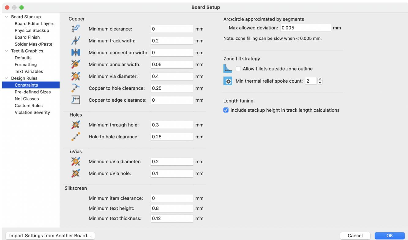
In addition to setting minimum clearances, a number of features can be configured here:
