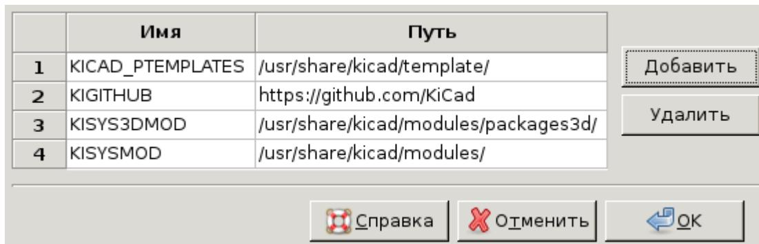
Paths set in the Configure Paths dialog are internal to KiCad and are not visible as environment variables outside of KiCad. They are stored in [KiCad's user configuration files](#).
